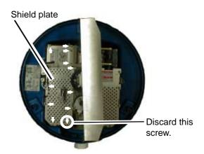
Antenna unit, cover removed, top view
